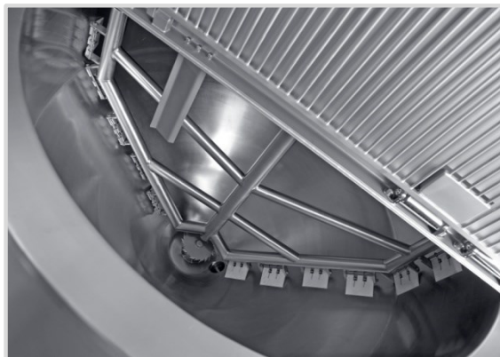
Inside view with dispersion and anchor type agitator
